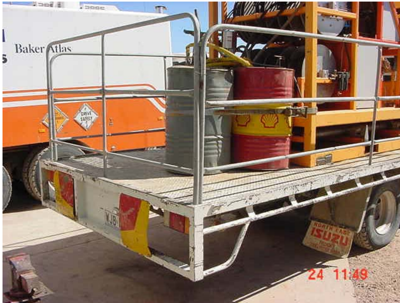
Truck Modified with Safety Rails
