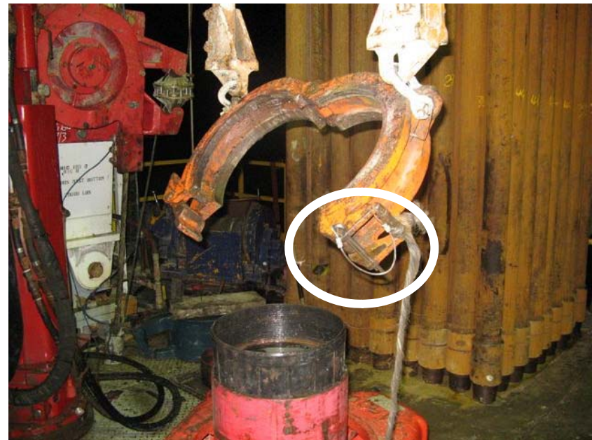
Immediately after the incident note safety pin still inserted.
