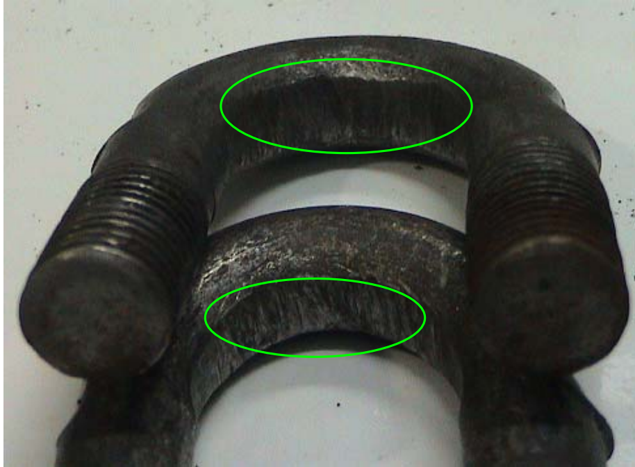
Figure 5 – U bolts showing signs of relative movement between the line and retainer. The lines are caused by gouging from the drill line. This is indicative of a problem with the clamp assembly or the installation of the clamp assembly
