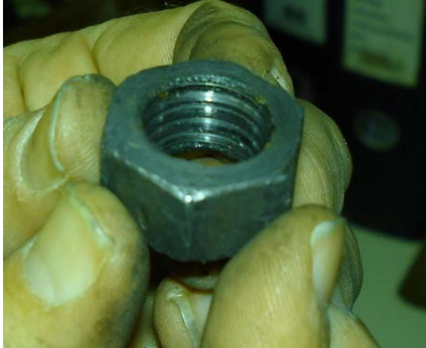
Figure 6 – Threads show signs of spalling. DO NOT USE
