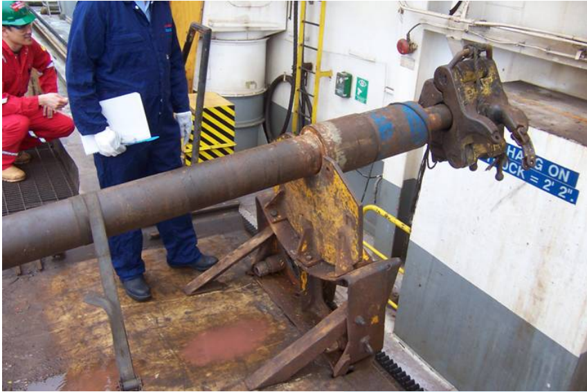
Tool position prior to impact (securing straps not in place at the time of impact)
